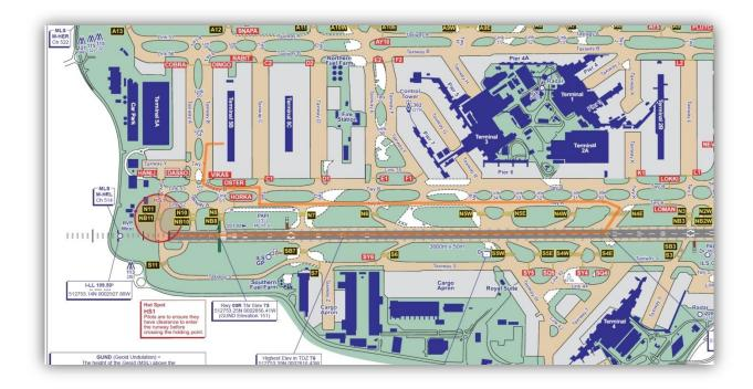
From our landing data, we can chose our autobrake setting to decelerate enough for N4E which is the taxiway we will use to vacate the runway. The best setting to do so is using Autobrake 3.
